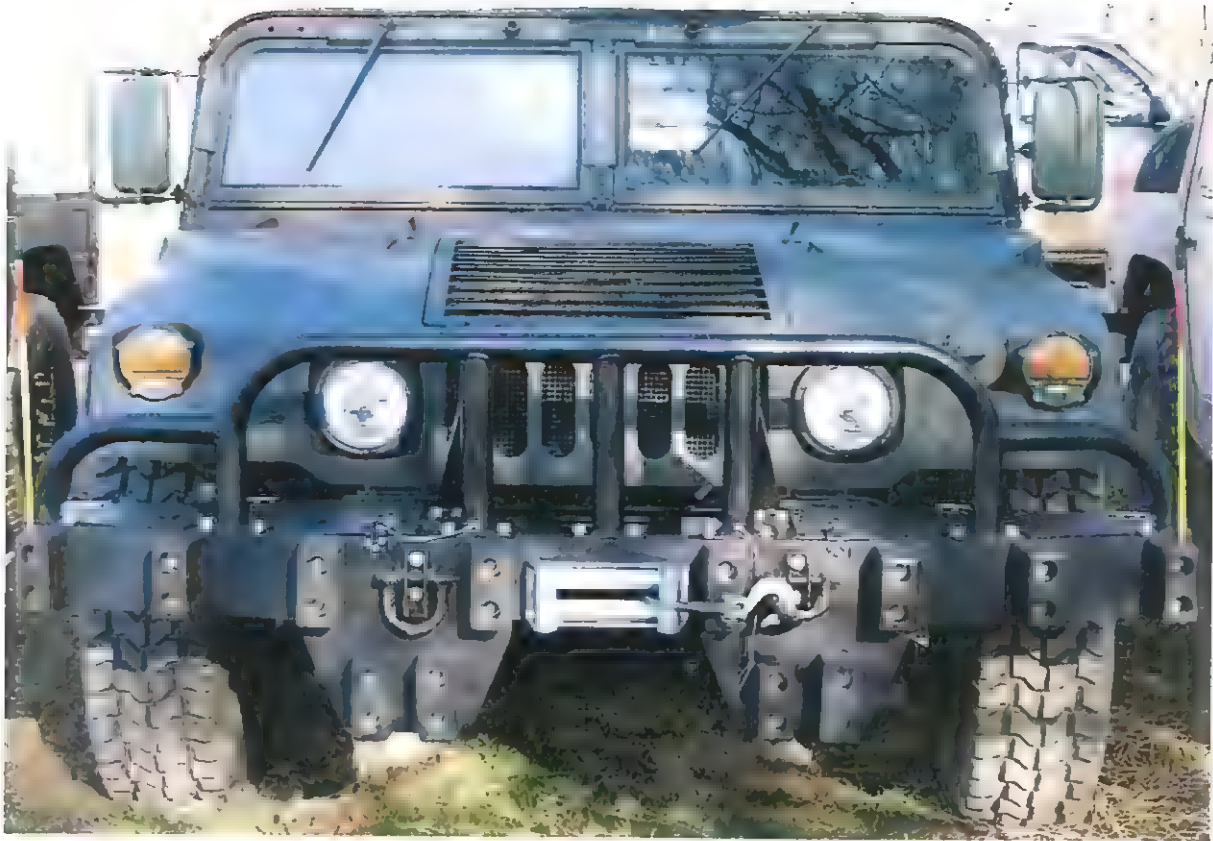
FIGURE 20. BUMPER (SHOWN WITH OPTIONAL VEHICLE PUSH ASSIST SYSTEM) INSTALLED ON M990 – SERIES HMMWV WITH WINCH KIT
