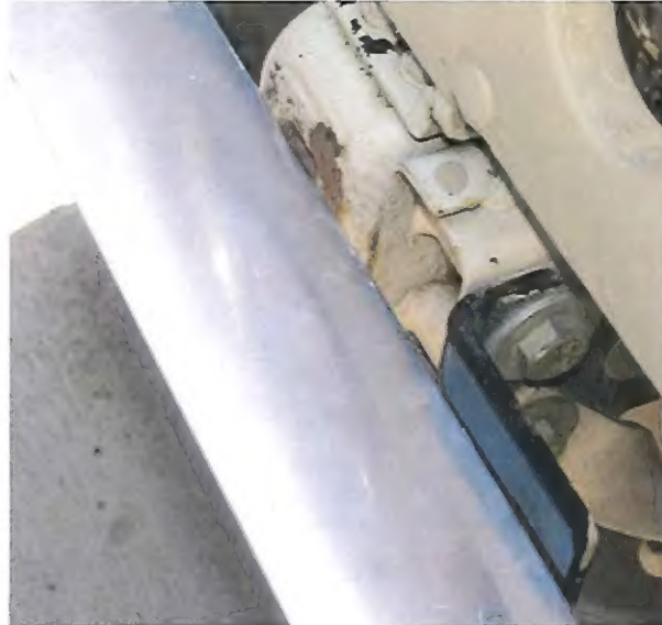
FIGURE 13. USE A STRAIGHTEDGE TO CHECK THE BRACKET
