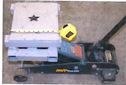
FIGURE 6. FLOOR JACK WITH LOCALLY-MADE SUPPORT PLATE
