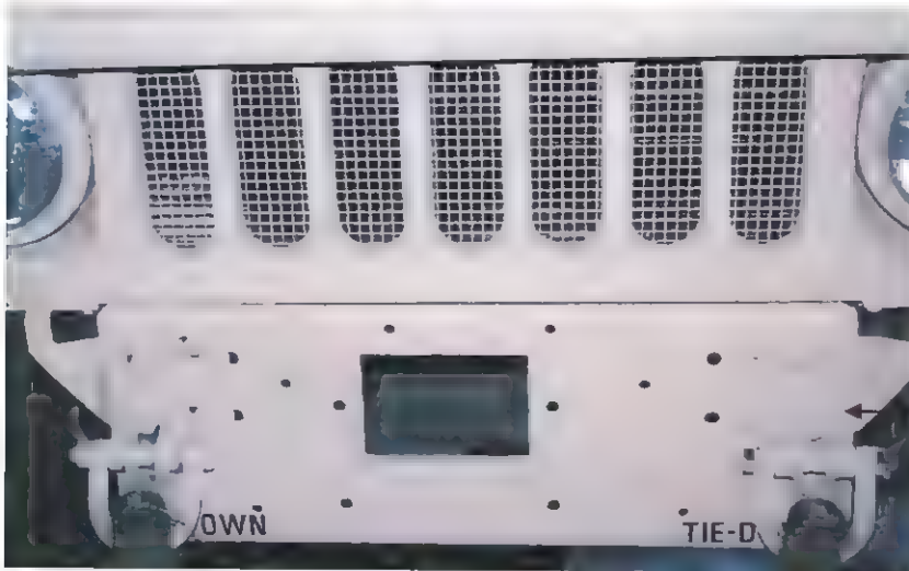
FIGURE 23. REMOVE LIFTING SHACKLES AND THEIR FOUR FASTENERS
