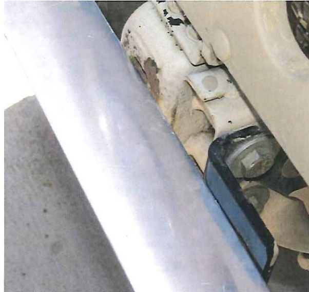
FIGURE 13. USE A STRAIGHTEDGE TO CHECK THE BRACKET
