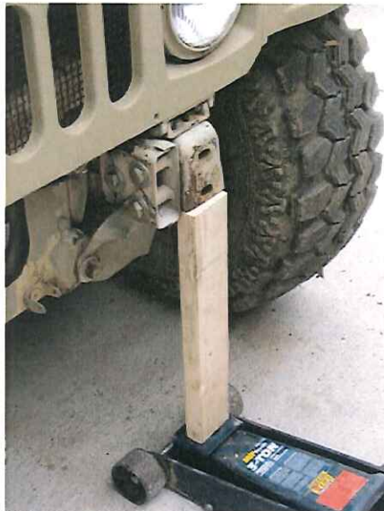
FIGURE 10. SUPPORT THE HOOD BRACKET WITH A FLOOR JACK
