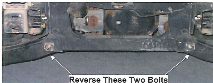
FIGURE 22. CONTROL ARM BOLTS REVERSED
