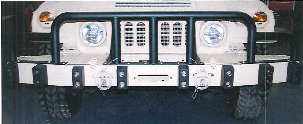
FIGURE 35. FPB INSTALLED ON M1114 HMMWV (REAR LIFTING SHACKLES NOT SHOWN)
