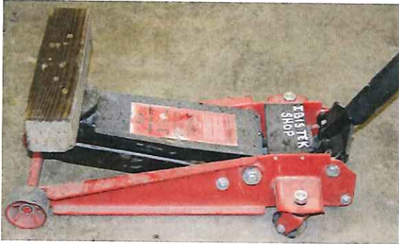
FIGURE 5. FLOOR JACK WITH 4" X4" BOARD
