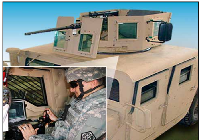
RSF enables remote operation of the turret while protected inside the vehicle
